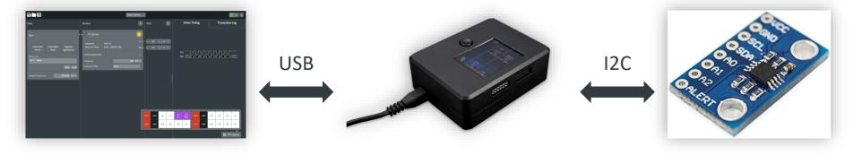
Readout Temperature sensor via FPGA (Efinix)
