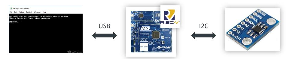
Readout emulated Temperature sensor via FPGA (Efinix)
