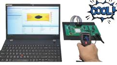
The photo shows the Ti375 running PCIe Gen4x4 and registering 29° C on a temperature monitor
