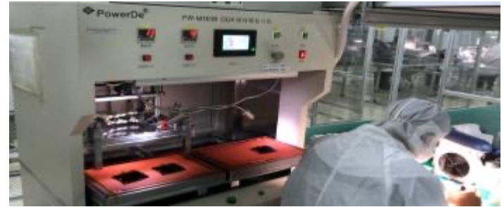
Automatic Optical Bonding Process of CTP on TFT
